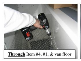
Attach to wood floor or rubber floor mat using #10 x 1" Phillips pan head sheet metal screws
